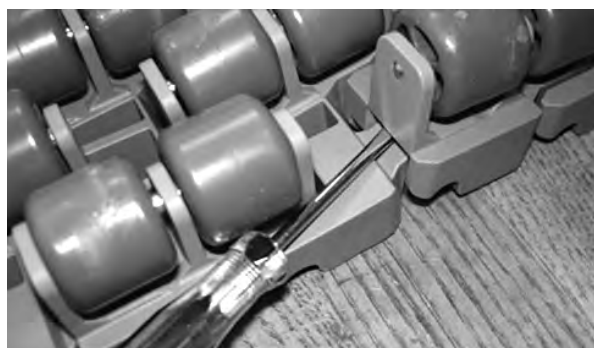
Figur 192: Sett inn skrutrekker under rullen
